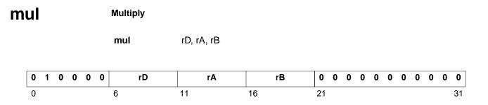
Multiplies the contents of registers rA and rB and puts the result in register rD. This is a 32bit by 32-bit multiplication that will produce a 64-bit result. The least significant word of this value is placed in rD. The most significant word is discarded.
